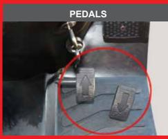
Hydrostatic control pedals for smooth handsfree forward & reverse motion (hst-models).
