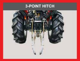
3-point hitch rear Category I provides a lift capacity of 650 kg.
