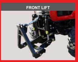
Frontlift cat. 0 with a lift capacity of 700 kg.
