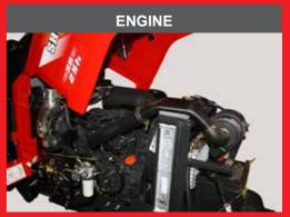
3-cylinder diesel engine delivers the highest power in its class with outstanding durability and reliability. The engines of SB22 and SB25 comply with the Stage V emission standard.
