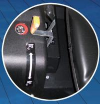
The mower on/off lever is located at the right side of the seat for ease of use.
