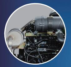
High-displacement, high-output Shibaura N843 Dieselengine that fulfills exhaust emissions regulations - 1496 cc engine of 28 HP power.
