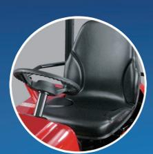
The Shibaura SG280 Slope mower will make the maintenance of steeply sloping grassed areas a lot easier, safer and more comfortable for the operator on the flat or slopes with its tilting seats to compensate for the working angle.
