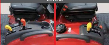
Various levers (HST Hi-Lo range shift, PTO select/clutch, etc.) are arranged either side of the operator seat in an optimal layout to ensure comfortable operation.
