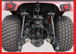
Combined with the rear PTO and category-1 three-point hitch, a variety of implements and attachments can be fitted according to the type of works.
