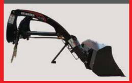
SPECIFICATIONS Maximum lift height to pivot pin: 1810 mm Maximum lift height under level bucket: 1638 mm Clearance with bucket dumped: 1298 mm Maximum dump angle: 45° Maximum rollback angle : 27° Dig depth: 130 mm Breakout force at bucket pivot pin: 604 kg Lift capacity to maximum height : 306.3 kg
