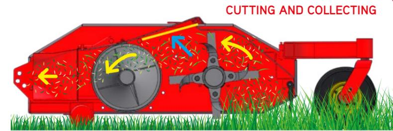
**GF3x1Plus**, through a small hydraulic cylinder operated using a practical button (on PG) and a practical manual lever (on TURBO1-2-4), it also makes it possible for the user to mulch.
