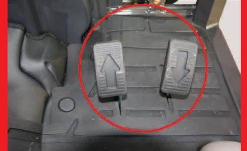
Hydrostatic control pedals for smooth hands free forward and reverse motion.
