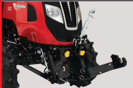
Front lift cat. 1 with a lifting capacity of 1000 kg.
