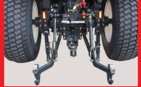
The category 1 hitch has a lift capacity of 1650 kg at the ball end.
