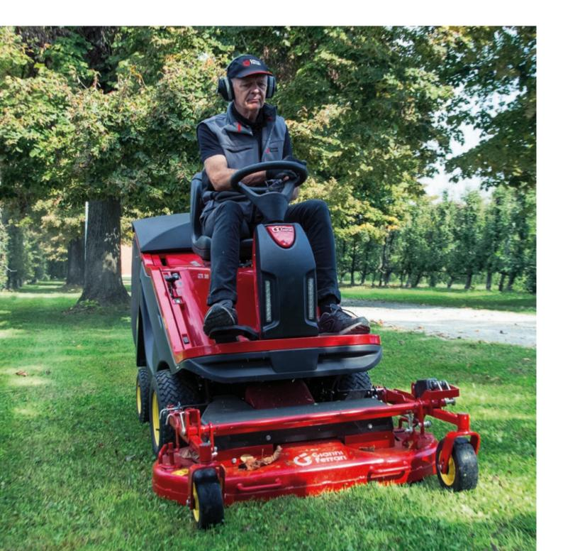
The deck offers a cutting width of 112 cm, is floating to naturally adapt to undulating terrain and is equipped with solid rubber anti-puncture wheels.
