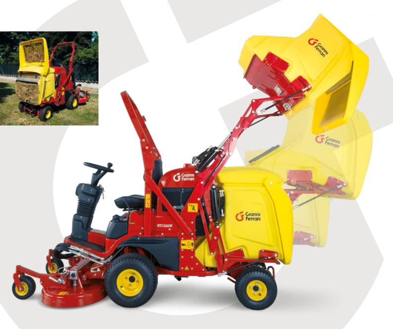
The collector is unloaded by operating a single **lever control**.
