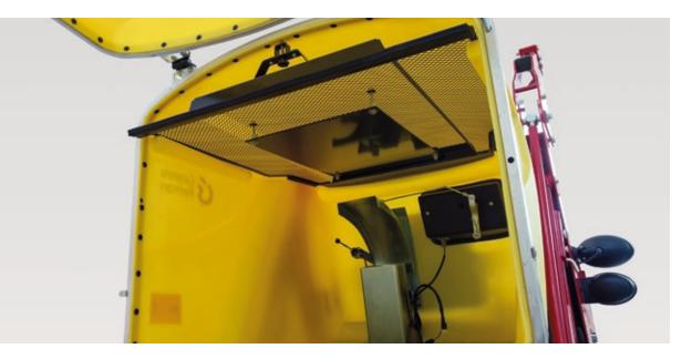
An efficient high-lift dump allows the operator to **easily and rapidly discharge the cut grass** directly into a truck or a trailer. The collector can optionally be equipped with a **dust filter** to minimise the exit of dust and collected material. Self-cleaning with electric motor for each disengaging of the suction turbine.
