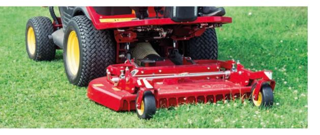
130 RCA mowers are distinguished by the direction of rotation of the blades, which is opposite to that of traditional mowers. The reverse rotation combined with the unique shape of the desk shell offer **excellent cutting quality** and a **high collection capacity** even with tall, wet grass. The **front opening of the deck**, equipped with mobile safety flaps, prevents the grass from over-bending for a more accurate cut.
