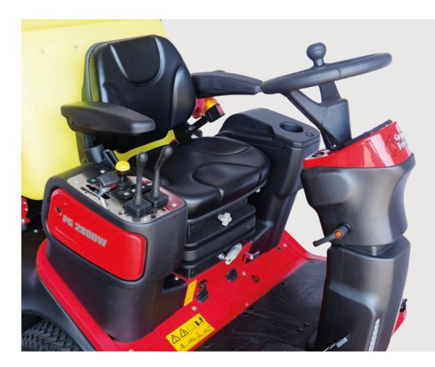
On the XPRO version, the main controls have been positioned to the right of the operator for greater convenience and ease of use. An LCD **dashboard** is available for the entire range for optimal machine management during use.
