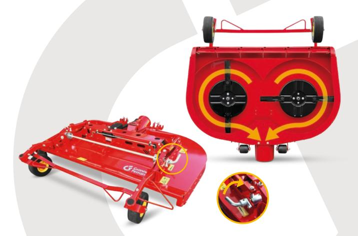
**Blade transmission** by mechanical reducers and helical bevel gears in an oil bath **is robust** and reliable.
