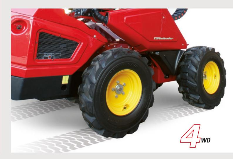
The **H440-2S** model is equipped with **4 dualspeed engines** to ensure maximum grip in slow drive and high transfer rates in fast drive. Turboloader is equipped as standard with a device that helps you get out of poor grip conditions. For more demanding situations, a hydraulic flow divider that replicates the operation of a mechanical differential lock is available as an option.
